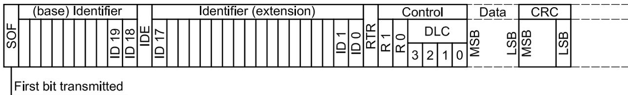
**Figure 11 — Order of bit transmission (extended format)**
