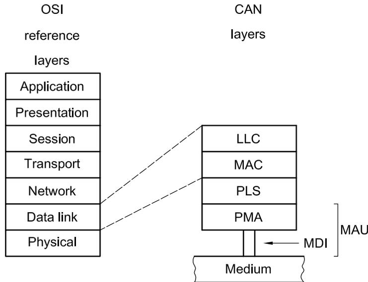
Figure 12 — Model of PL architecture
