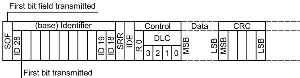
**Figure 10 — Order of bit transmission (base format)**
