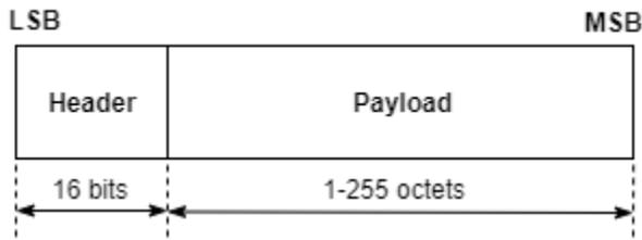
The advertising physical channel PDU has a 16-bit header and a variable-size payload. The 16-bit header field of the advertising physical channel PDU is shown in this figure.
